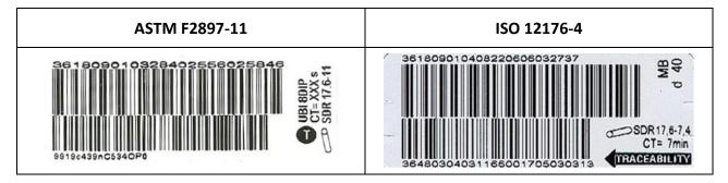
The Pipe/Fitting Traceability option can only be enabled through the Features Menu (see page 29). When this option is set to "ON" or "OPT", in addition to the fitting barcode, the operator will be prompted to scan one or more traceability barcodes that are attached to the pipe and/or the fitting. This data will not affect the fusion; however, it will be associated with the fusion in the download.
